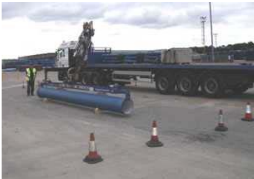
Individual pipes are secured to the beam by a hydraulic locking system, as shown in this picture
