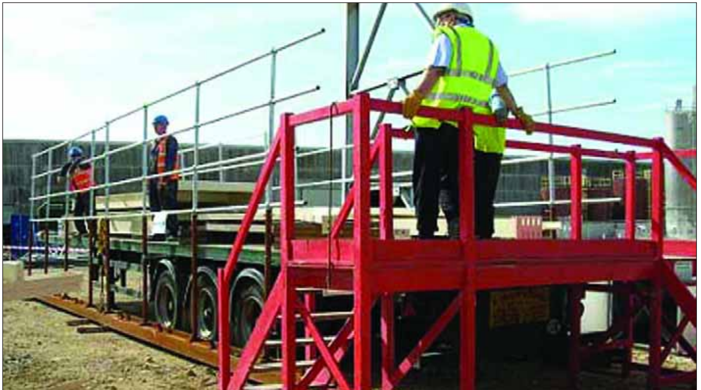
Figure 1 Trailer edge protection system with access platform and steps
