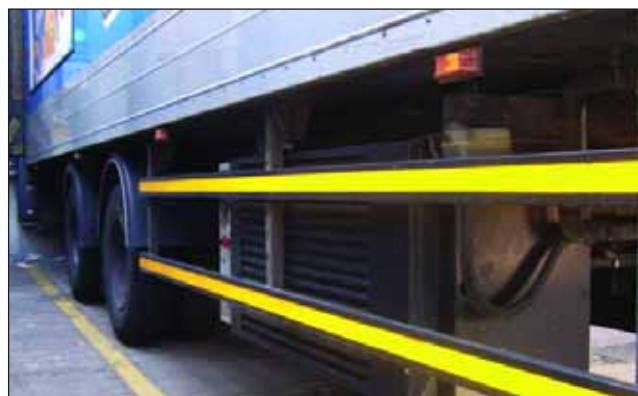
Figure 2 Under-slung refrigeration unit
