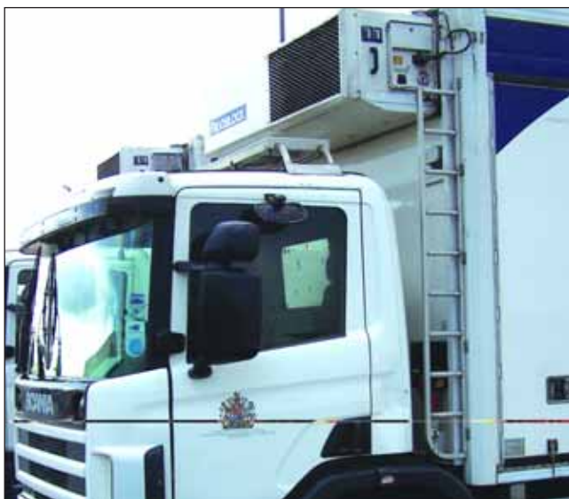
Figure 1 Access ladder to refrigeration equipment on old vehicles
