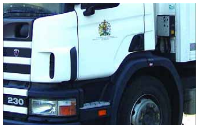
Figure 2 New controls at ground level eliminating the need for a ladder.
