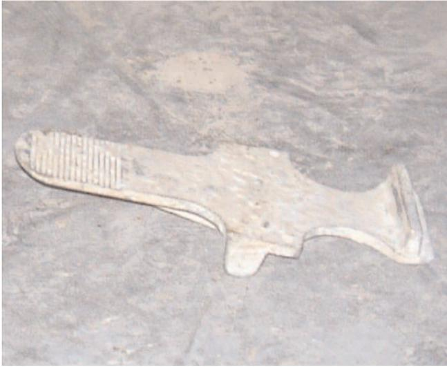
*Figures 3 and 4 Board lifting tool*
