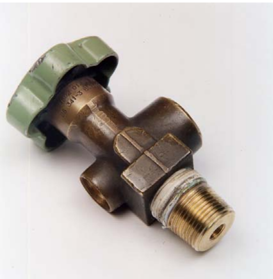
Markings can be obscured by valve handle
