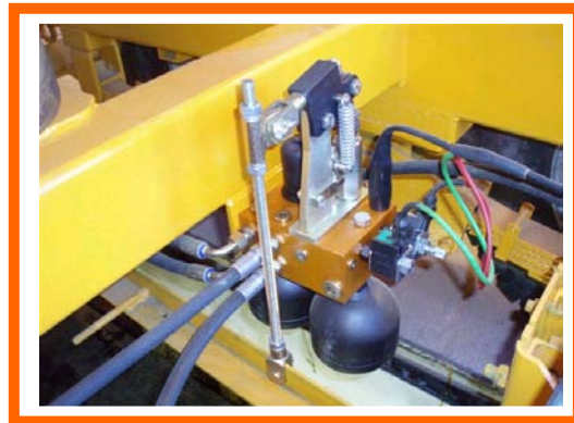
Fig.2 Hydraulic combined fail-safe emergency load sensing valve
