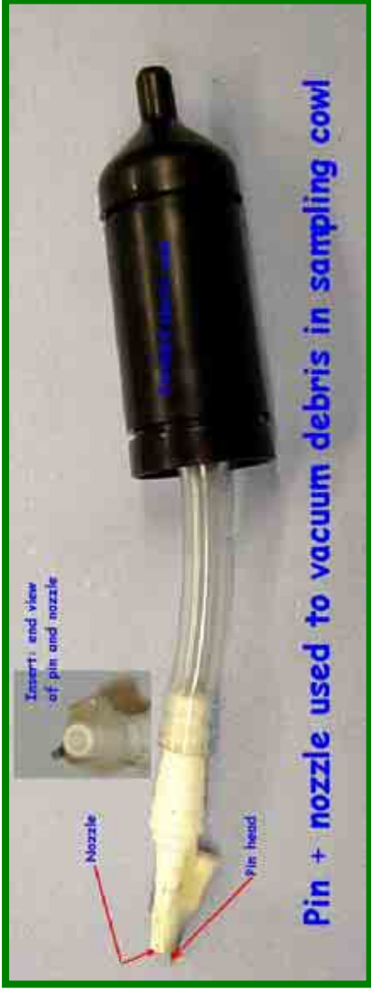
Figure 2: Photograph of device used to hold the point of the pin in front of the nozzle used to vacuum debris into a standard sampling cowl.
