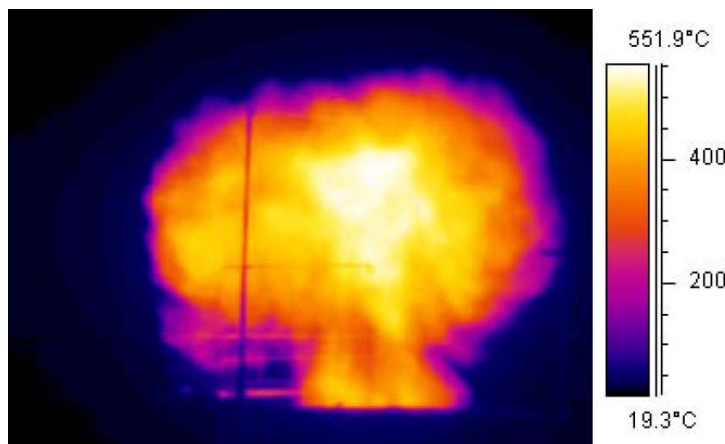
venting of hydrogen deflagration from a roof vent
