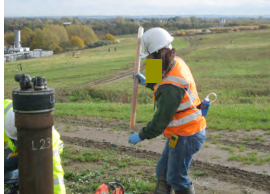
Figure 8 Sampling the leachate
