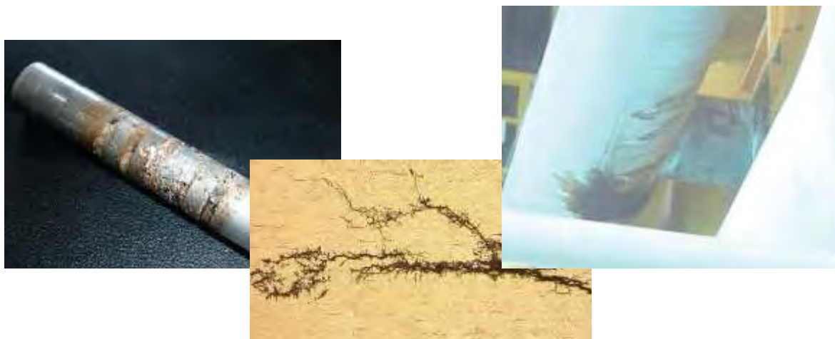
Figure 7: Examples of Stress Corrosion Cracking
