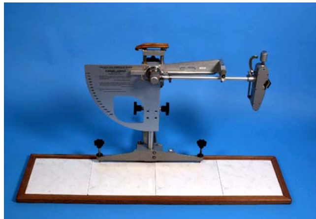
Figure 2.2 Slipperiness assessment test methods; the “Stanley” Pendulum CoF test.
