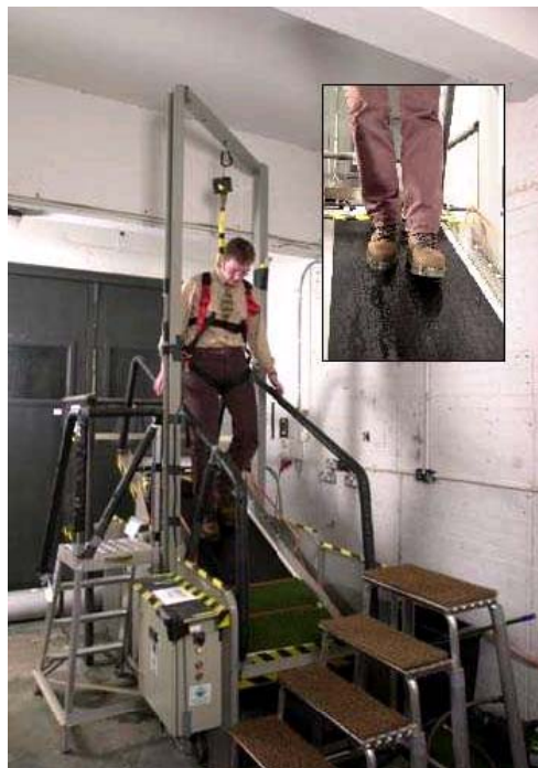
Figure 2.3 The ‘HSL-PS-SOP-12’ ramp-type CoF test.
