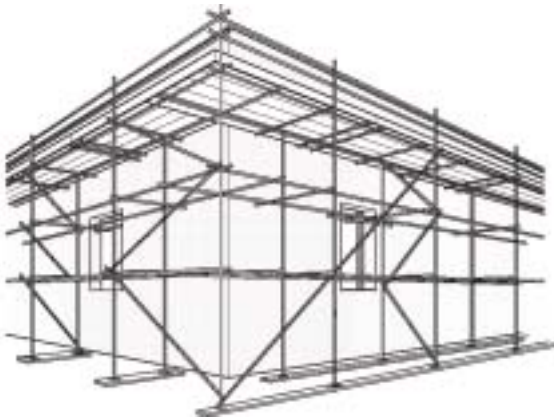
Typical independent tied scaffolding.
