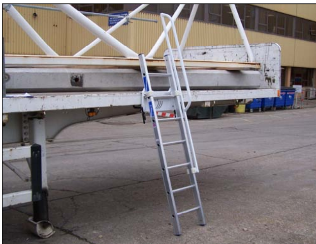
Figure 1 Ladder in use on flat-bed trailer
