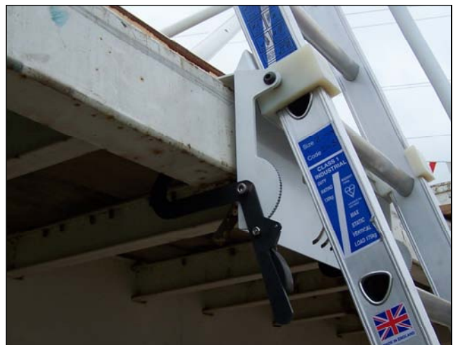
Figure 2 Showing ratchet clamping system
