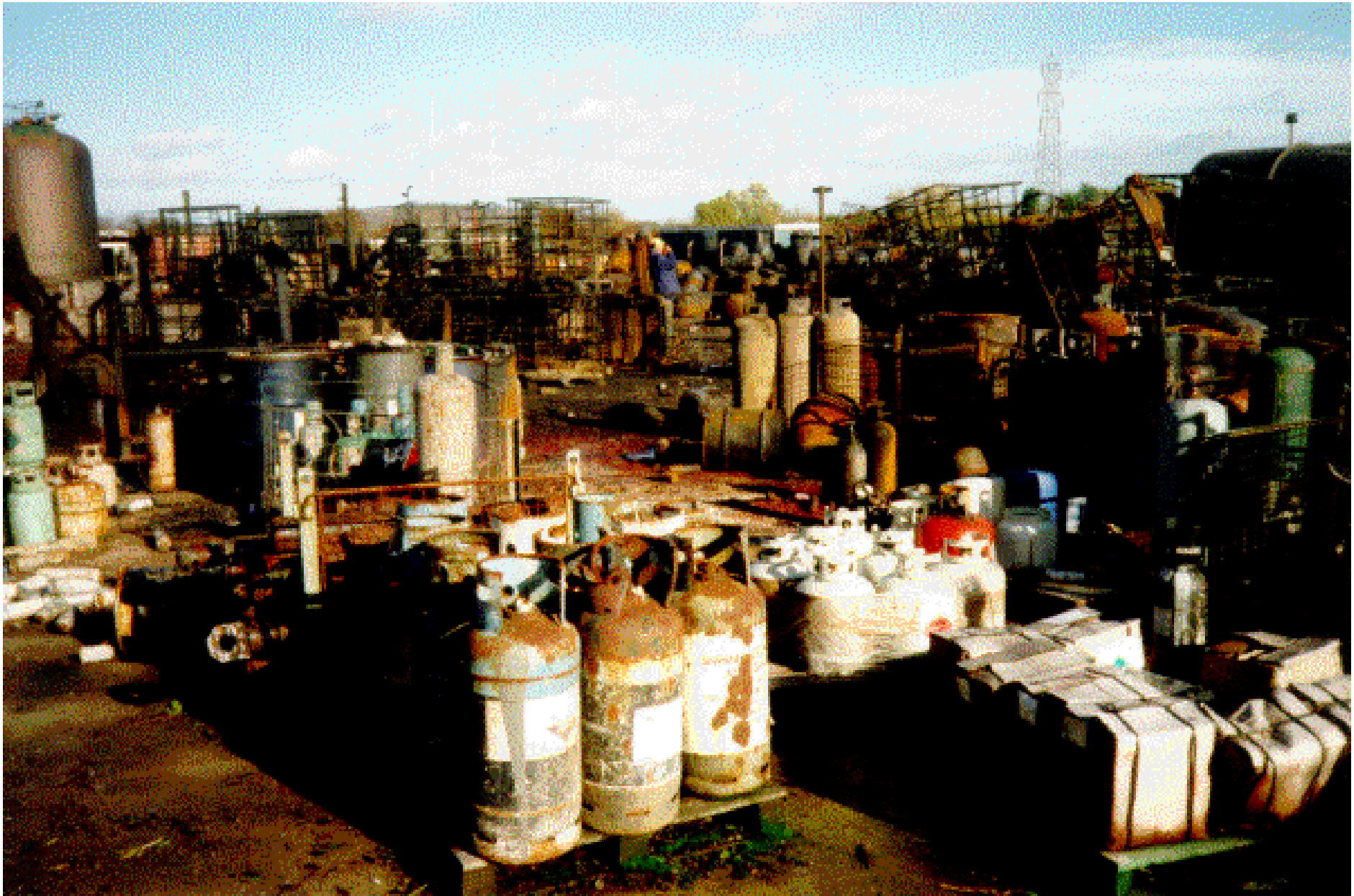
Photograph 3: Close up of compound 3 after the fire showing fire damaged cylinders.
