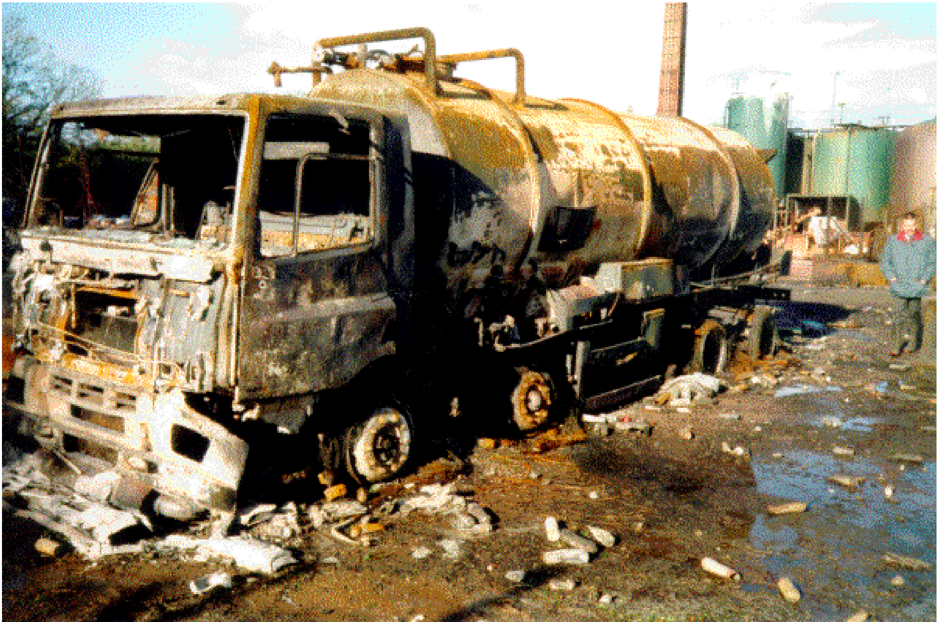
Photograph 4: Close up of compound 3 after the fire showing fire damaged tanker.
